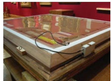
11. The back of a 'conservation framed' painting. This shows the an embedded sensor/telemetric logger that records and transmits relative humidity and temperature data back to the Conservation Dept every 30 minutes. Together with the glazing at the front, the impermeable polyester film membrane sealing the back creates a microclimate around the painting.
